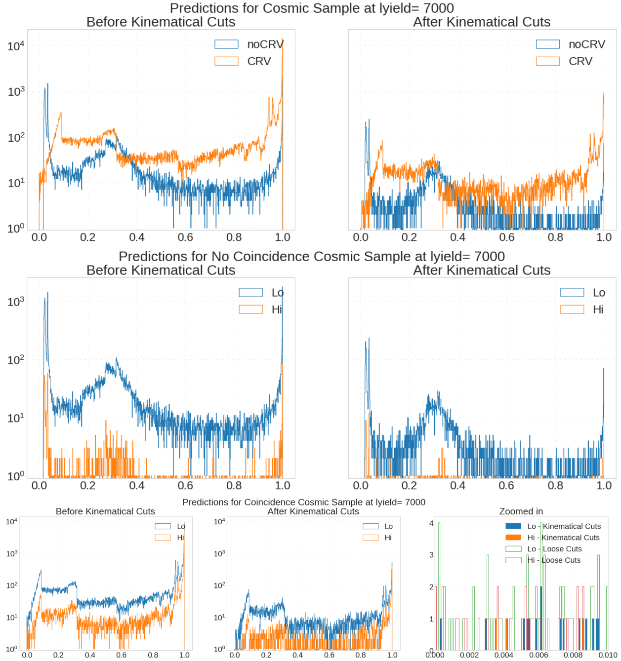
Figure 22: Predictions for the subset of the CRY4 sample that has a lightyield of 7,000. “Lo” (in blue) indicates low energy muons, and “Hi” (in orange) indicates high energy muons for the plots in the middle and bottom.
